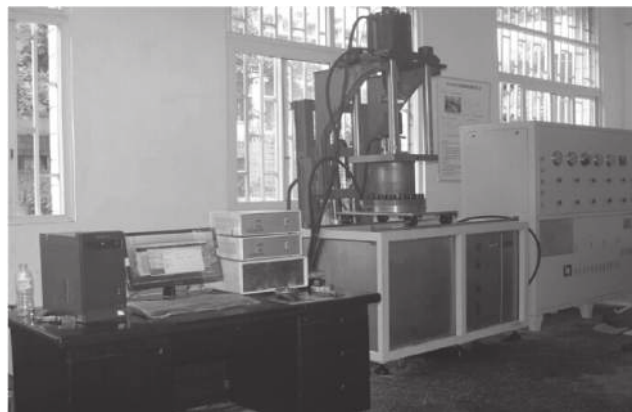
Fig.5 Experimental setup for coupled fluid flow and dissolution test for salt rock fracture
