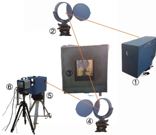
①-Light; ②-Speculum I; ③-Protective box (Flow field area); ④-Speculum II; ⑤-Light source receiving box; ⑥-High-speed camera
