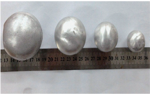
图 1 铸造法制备的可溶性镁合金 Fig. 1 Soluble magnesium alloy prepared by casting
