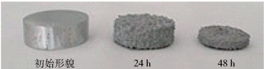
图5 可溶性镁合金浸泡前后形貌 Fig.5 Morphology of soluble magnesium alloy before and after immersion
